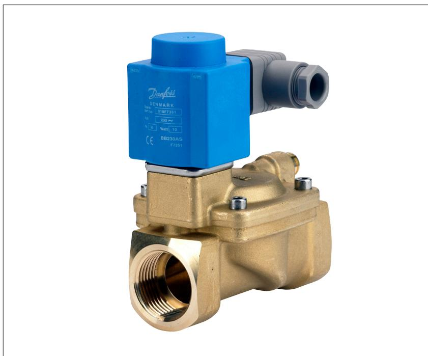
EV220B 15 – EV220B 50 is a universal indirect servo-operated 2/2-way solenoid valve program. Valve body in brass, dezincification resistant brass and stainless steel ensures that a broad variety of application can be covered. Built-in pilot filter as standard, adjustable closing time and enclosures up to IP67 ensures optimal performance even under critical working conditions.
