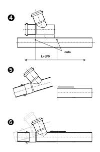
Both pipe ends are trimmed and slanted. A sleeve socket is then pushed over one end and the other pipe end is cautiously levered out, the branch is pushed on 6 and the end of the pipe with the branch is brought back into the original position. The connection is made by means of pushing back the sleeve socket on the cut between the pipe and the fittings spigot end 6.
