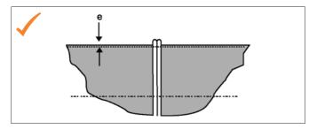
Illustration 5.7 Butt-weld with even welding beads (acceptable)
