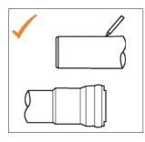
*Plug-in socket:* The pipe needs to be inserted in the plug-in socket using the full insertion depth.
