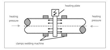
Illustration 5.5 Obtaining the correct heating depth
