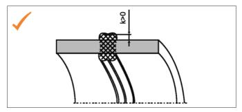
Illustration 5.11 Cross section of a good butt-weld
