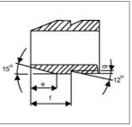
The pipe end needs to be chamfered under an angle of 15°. The groove needs to be cut under an angle of 12°. The correct dimensions can be found in table 5.5. To get an even cut and chamfer it is recommended to use an Akatherm groove cutter.
