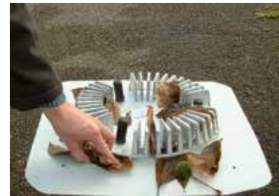
Ensure the leafguard grid is in place. Clean the leafguard grid.
