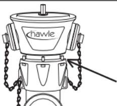
loosen the bolts, remove the head
