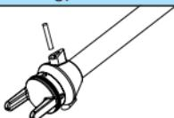
take out the operating controls, change the valve plug\*, insert the operating control
