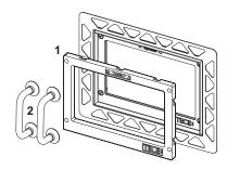
9820196 Toilet support frame for flush-mounted installation
