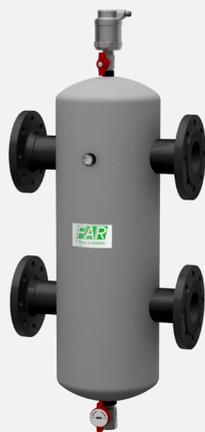
Hydraulic separator complete with flanged connections, automatic air vent valve with shut-off valve, drain cock and anti-condensation insulation.
