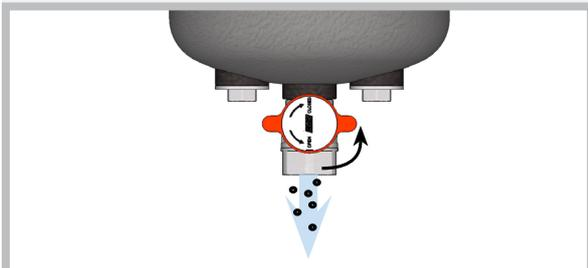
In the event of leakage from the air vent valve it is necessary to clean or replace it. Once the ball valve is closed, the air vent valve can be unscrewed by means of a 4mm Allen wrench. Unscrew the stem to proceed with cleaning or replacement.
