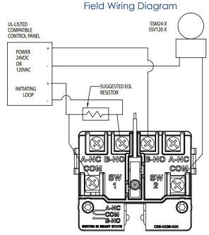
NOTE: COMMON AND B-NO CONNECTIONS WILL CLOSE WHEN VANE IS DEFLECTED, LE, WHEN WATER IS FLOWING, DUAL SWITCHES PERMIT APPLICATIONS TO BE COMBINED ON A SINGLE DETECTOR.
