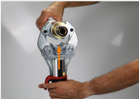
For a correct position of the press jaws on the fitting, the outer jaws pair encloses the fitting fully.
