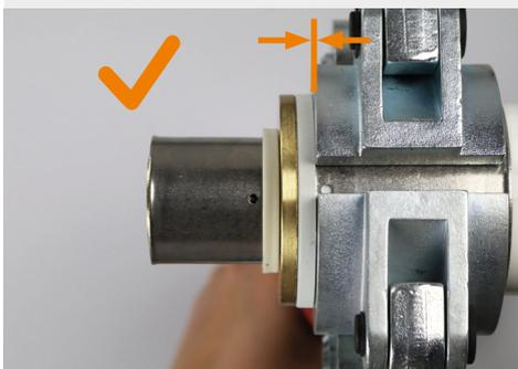
It is important to ensure that all three parts of the press jaws are rectangular and flush to the fitting.
