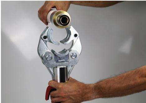
Open the press jaws by pushing the axle stub between thumb and index finger.
