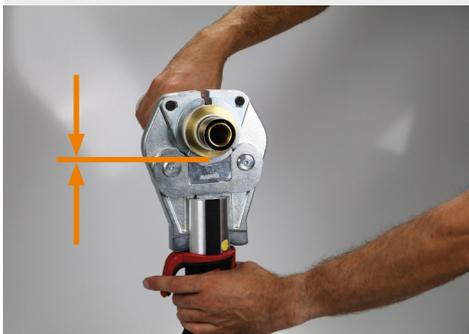
Subsequently, the pressing machine, with the third lower press jaws part, is brought into contact with the sleeve by pushing the fitting towards the machine. The fitting is then enclosed by all three parts of the press jaws.
