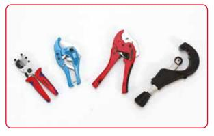
A range of cutter types are available to suit the pipe diameter.
