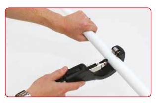
Use a set of Maincor disc type cutters for pipes larger than 32mm.
