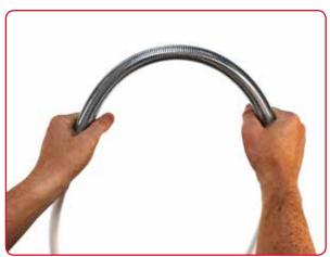
Bending the pipe using an External Bending Spring.
