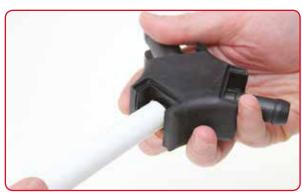
Prior to fitting connectors, the pipe is to be bevelled by inserting the bevelling tool and rotating the tool three full turns. This will put a 45° chamfer on the pipe and the pipe will be ready to take the fitting.
