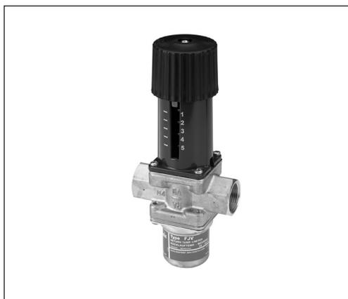
The FJV ensures that return water is cooled to required temperature before it flows back to the district heating plant. Controller closes on rising temperature.
