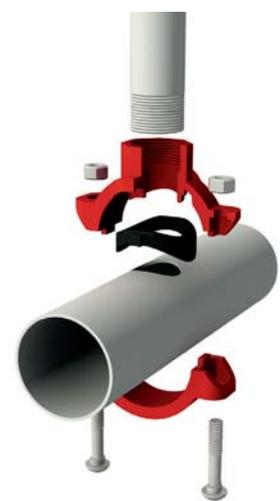
Care should be taken to maintain the area of around 16mm outside the hole (quota s), along with the section of the tube of length L, free of burr, grease, dirt etc., with the aim of achieving total sealing. The coupling should sit perfectly.
