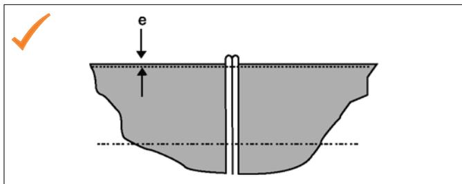
Illustration 5.7 Butt-weld with even welding beads (acceptable)
