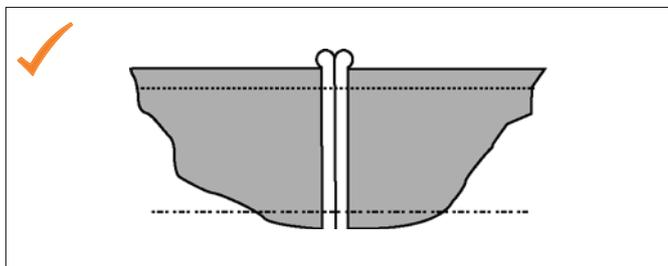
Illustration 5.9 Butt-weld with big welding beads (acceptable)
