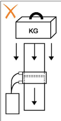
An additional load on the vertical pipe will transfer extra HDPE material to the fusion zone. This will cause movement of the wires and possibly a short circuit and thus a bad weld or fire hazard.
