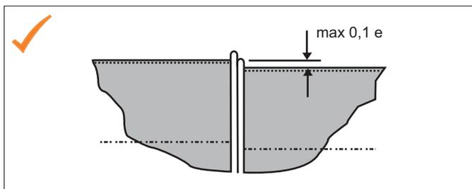
Illustration 5.8 Butt-weld with mis-alignment of pipe (acceptable)
