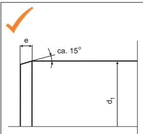
The pipe-end needs to be chamfered under an angle of 15°. A chamfering tool should be used to get an even cut and chamfer.
