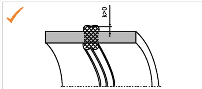
Illustration 5.11 Cross section of a good butt-weld
