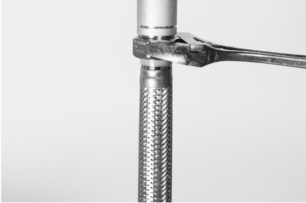
4. Bend the flexible hose to achieve the required routing maintaining the minimum bend radius and position the reducer for sprinkler location. When bending the hose allow 65mm of straight hose from the nut, ensure there are no kinks and use the Rapidrop Minimum Radius Indicator if required by Authority having Jurisdiction.
