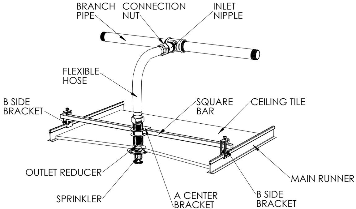
1. Install the Inlet Nipple in the Branch Pipe outlet using the normal sealing and tightening methods for connecting pipe threads. Tighten firmly with a pipe wrench for leak proof connection. For SPW this inlet nipple is permanently fixed to the flexible hose and care must be taken not to twist the hose or use it as a lever when tightening in the nipple.
