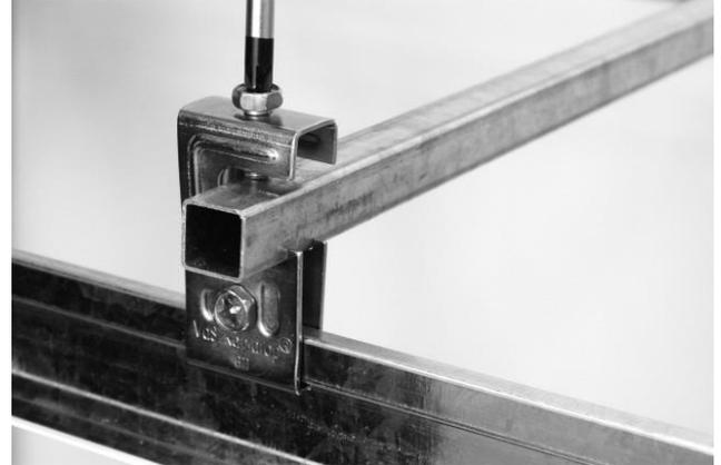
7. Slide A centre bracket onto the square bar, mount the outlet reducer through the A centre bracket and lightly tighten the nut. Adjust location of the centre bracket and the side B brackets until desired location of the outlet reducer is achieved. Firmly secure the side B brackets by tightening the screws to a torque of 5 Nm/4 ft-lbs.
