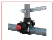
Tighten the bolts crossways. Use the tightening torque specified in the instruction manual. Connect the branch. Make sure there is no water in the branch when the T-plus is activated.
