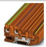
Sensor/actuator terminal block, with protective conductor function, nom. voltage: 250 V, nominal current: 20 A, connection method: Push-in connection, number of connections: 3, cross section: 0.2 mm² - 4 mm², AWG: 24 - 12, width: 7 mm, color: orange, mounting type: NS 35/7,5, NS 35/15
