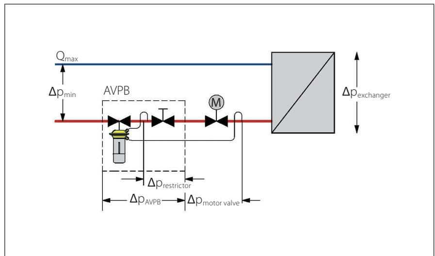
FIGURE 5: Differential pressure control and flow limitation of a heat exchanger system in a district-cooling network.
