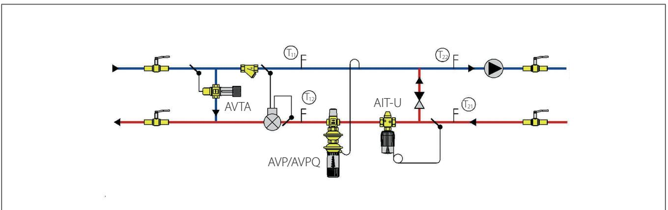
FIGURE 8: Self-acting control of a district cooling substation.
