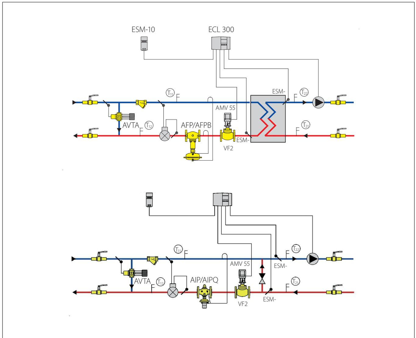
**FIGURE 9: Electronic control of a heat exchanger (above) and a mixing loop (below) in a district cooling system.**
