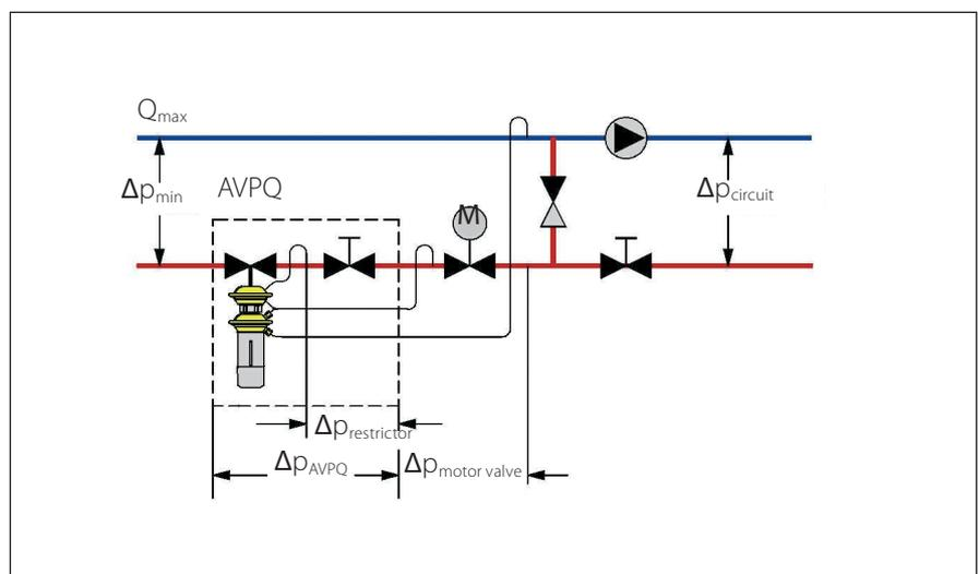
FIGURE 6: Combined differential pressure and flow control of a mixing loop in a district cooling system.
