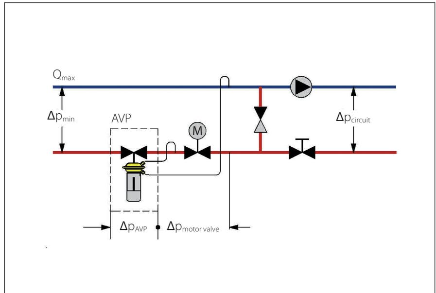
FIGURE 4: Differential pressure control of a mixing loop in a district cooling system.
